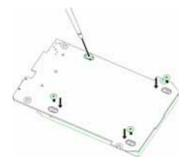
5 Place the printed circuit board/hard drive assembly into the enclosure with the hard drive face down, then secure it into the enclosure with the screws (4) you previously removed.
